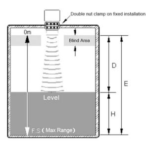
E ---The total face height of container to the sensor, that is the actual installation height.
