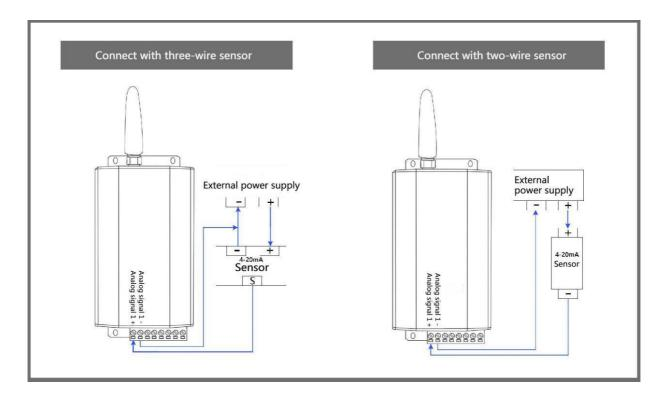
\*Note: When using RTU external power supply output port instead of external power supply to provide power for 4-20mA, 0-5V sensors and pin 8 is the positive pole of the power supply, and pin 7 is the negative.
